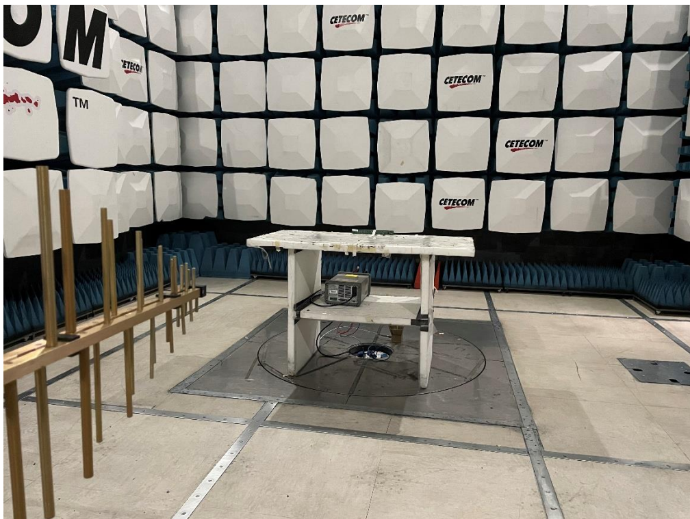
Photo 2: Emissions in frequency range 30 MHz to 1 GHz
