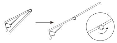
Assembling: Put the frame in the base with "  $\bigcirc$  " shape components aligned. Disassembling: Press the sheet metal and pull up the seat frame.
