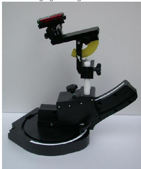
Device holder supplied by SPEAG
