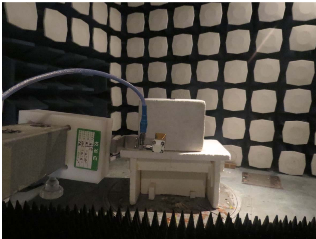
Picture 1 Radiated Emission Test Setup
