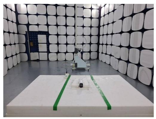
Radiated Emission (Below 30MHz) Powered by adapter
