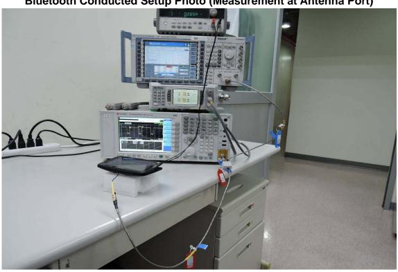
**BLE & WLAN Conducted Setup Photo (Measurement at Antenna Port)**
