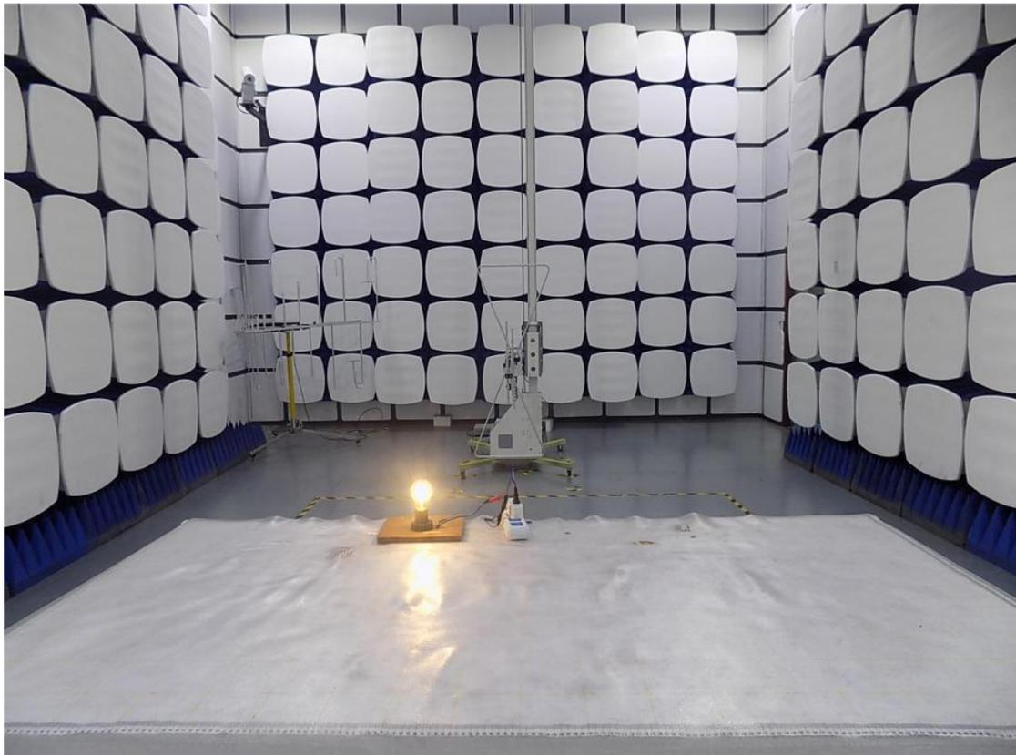
2.Setup for Radiated Emission above 1GHz
