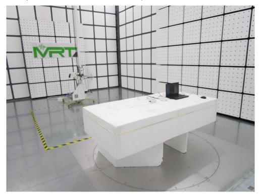
Description: Radiated Emission Test Setup for 1~18GHz
