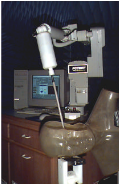
Figure 5. Photograph of the Probe and the Phantom
