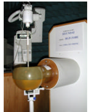
Figure 1. SAR Test Set-up
