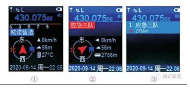
In standby mode, press the left and right arrows to switch the standby display
