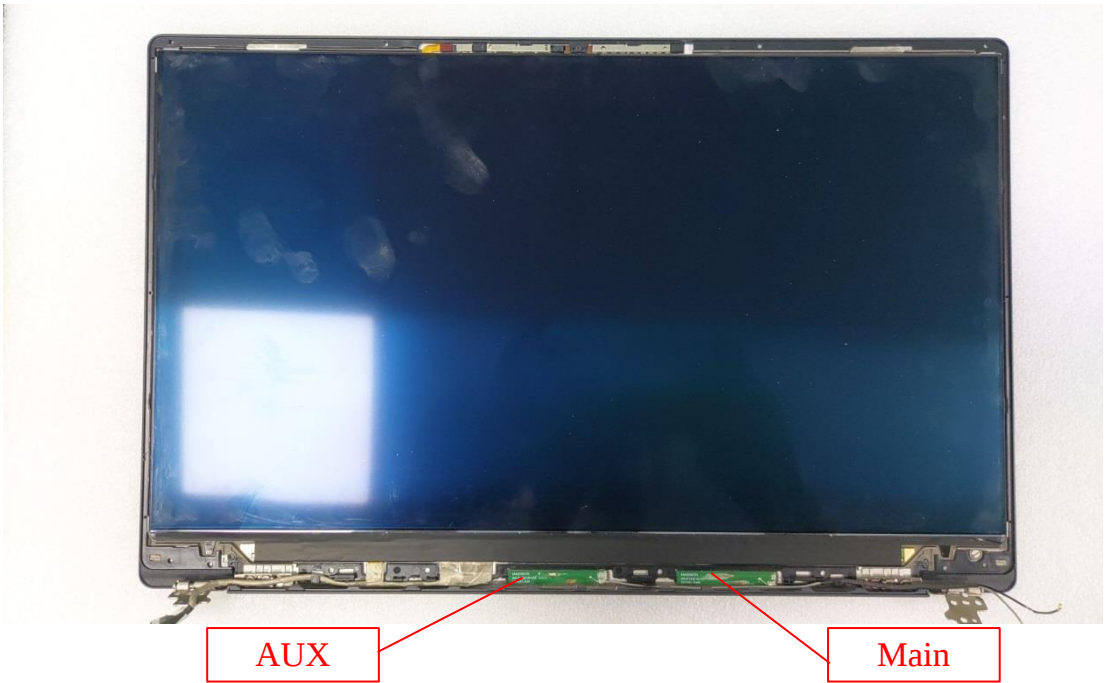
Figure 30 WLAN Combo Antenna (Main Black / AUX Gray)
