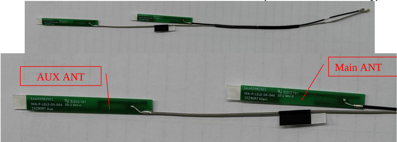
Figure 30 WLAN Combo Antenna (Main Black / AUX Gray)
