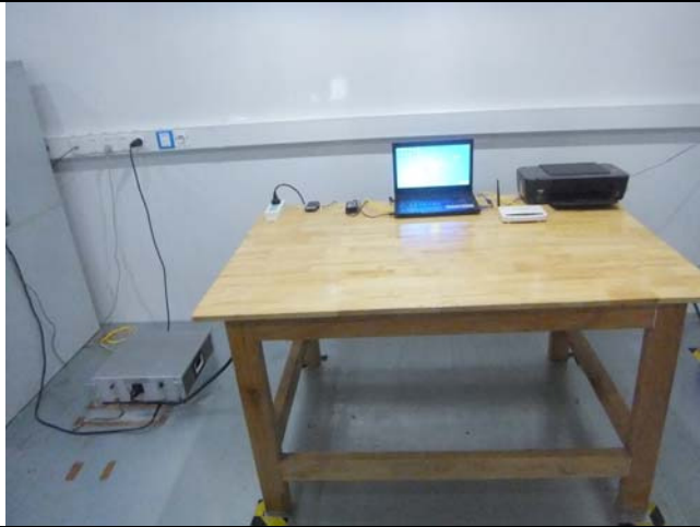
Conducted Emissions Test Setup – Front View
