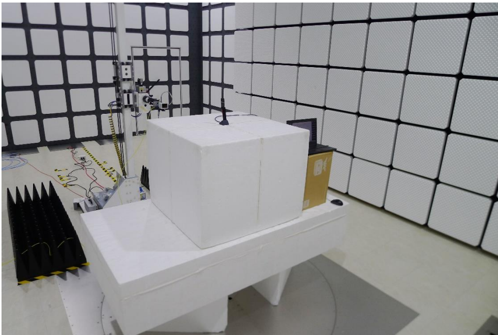
Description: Radiated Emission Test Setup for 18GHz~40GHz
