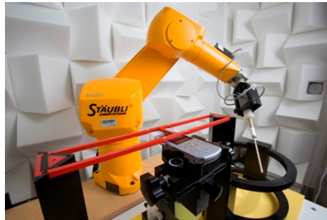
Figure 4-3 SPEAG Robotic System
