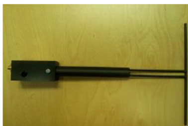
Figure 1 – MVG COMOSAR Validation Dipole
