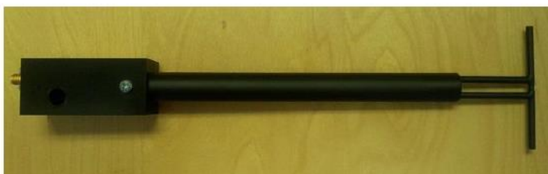
Figure 1 – MVG COMOSAR Validation Dipole
