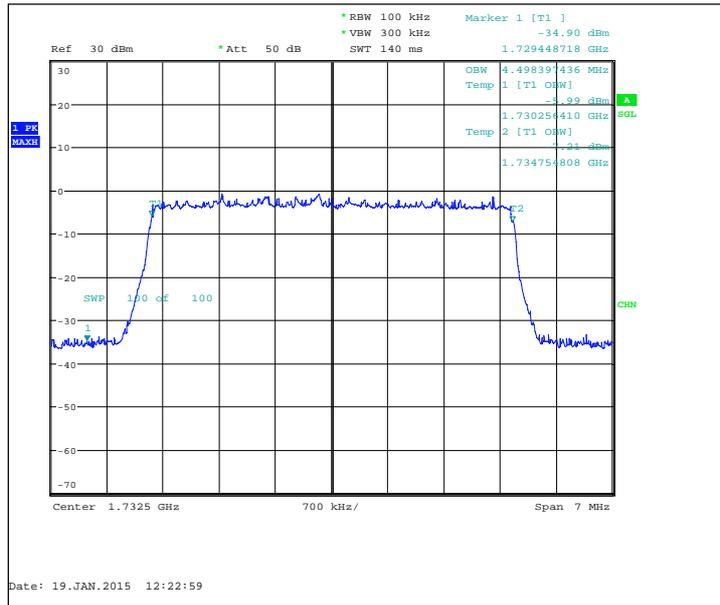
FDD, CBW 10MHz, QPSK, 50 RB, Channel 20175 / 1732.5 MHz
