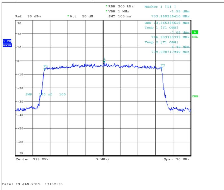
FDD, CBW 20MHz, QPSK, 100 RB, Channel 27435 / 725.5 MHz
