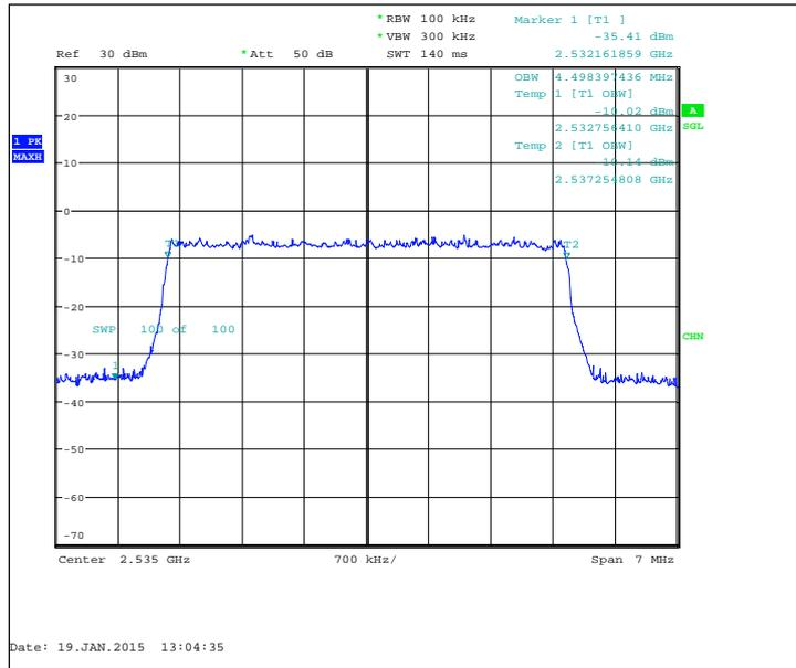
FDD, CBW 10MHz, 16QAM, 50 RB, Channel 21100 / 2535.0 MHz
