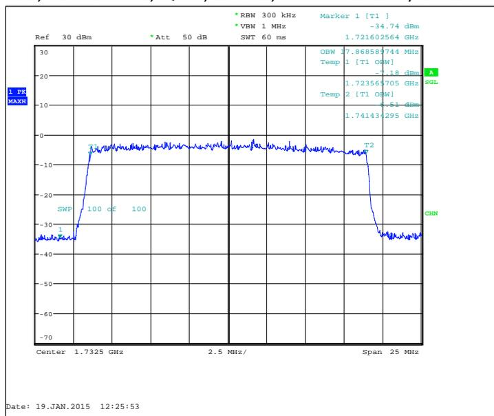
FDD, CBW 1.4MHz, 16QAM, 6 RB, Channel 20175 / 1732.5 MHz
