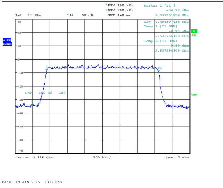
FDD, CBW 10MHz, QPSK, 50 RB, Channel 21100 / 2535.0 MHz
