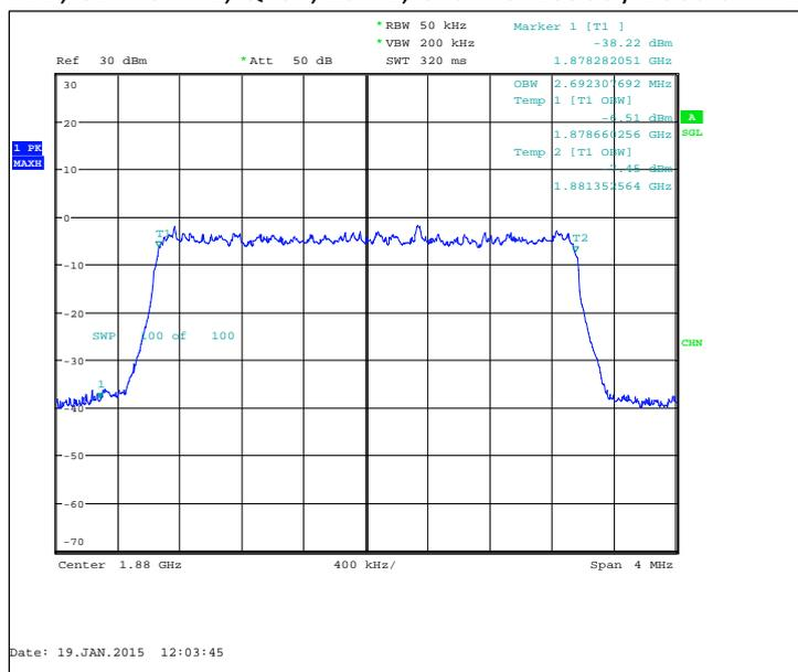
FDD, CBW 5MHz, QPSK, 25 RB, Channel 18900 / 1880.0 MHz
