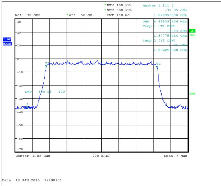
FDD, CBW 10MHz, QPSK, 50 RB, Channel 18900 / 1880.0 MHz
