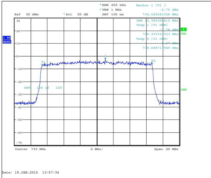
FDD, CBW 20MHz, 16QAM, 100 RB, Channel 27435 / 725.5 MHz
