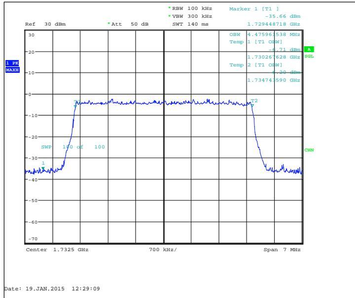
FDD, CBW 10MHz, 16QAM, 50 RB, Channel 20175 / 1732.5 MHz
