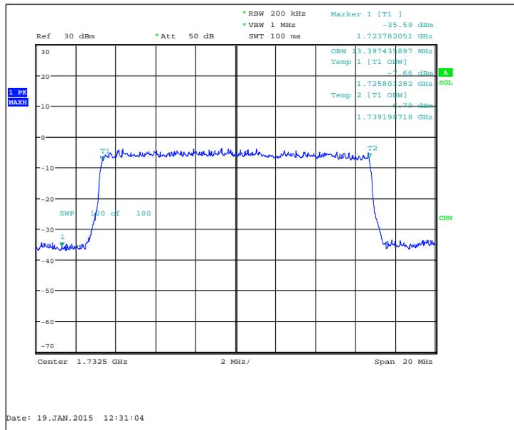
FDD, CBW 20MHz, 16QAM, 100 RB, Channel 20175 / 1732.5 MHz
