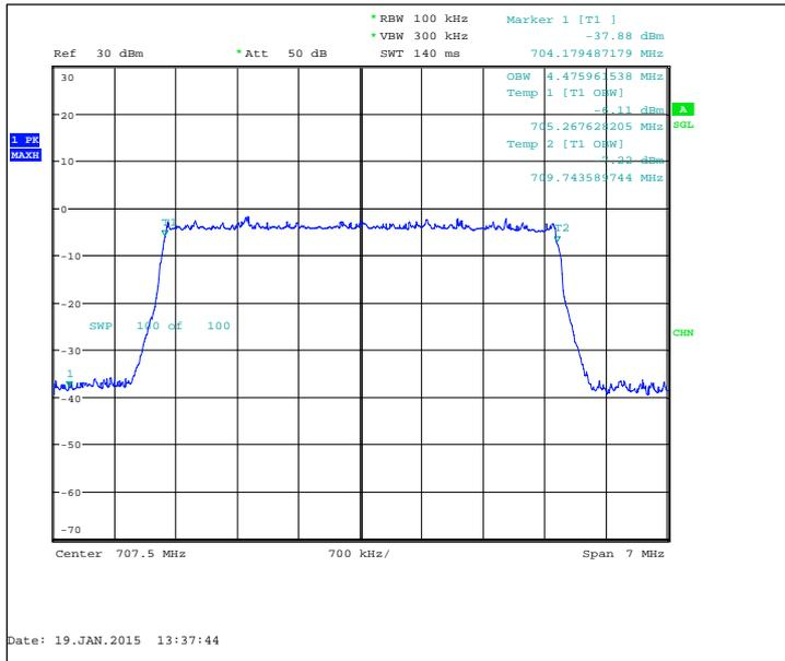
FDD, CBW 10MHz, 16QAM, 50 RB, Channel 23095 / 707.5 MHz
