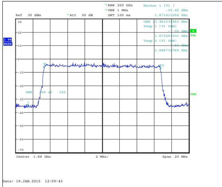
FDD, CBW 20MHz, QPSK, 100 RB, Channel 1890 / 1880.0 MHz
