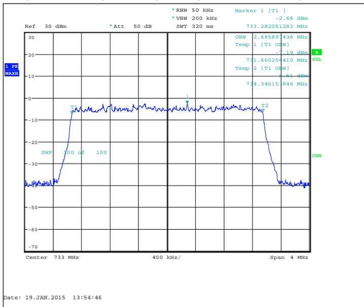
FDD, CBW 5MHz, 16QAM, 25 RB, Channel 27435 / 725.5 MHz
