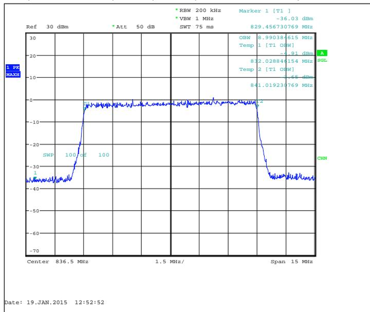
FDD, CBW 1.4MHz, 16QAM, 6 RB, Channel 20525 / 836.5 MHz
