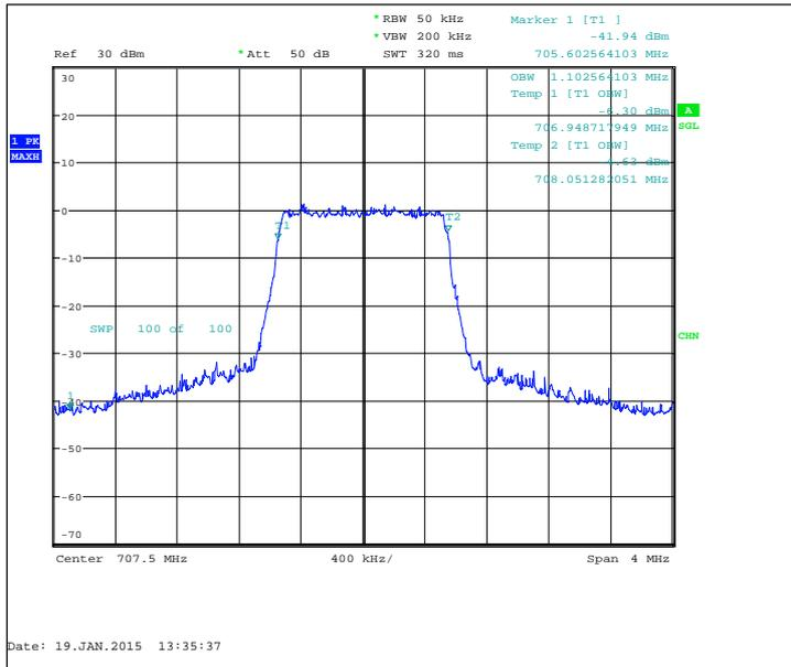
FDD, CBW 3MHz, 16QAM, 15 RB, Channel 23095 / 707.5 MHz
