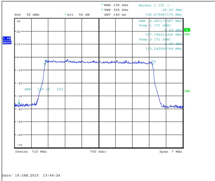
FDD, CBW 10MHz, 16QAM, 50 RB, Channel 23790 / 710.0 MHz
