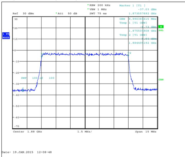
FDD, CBW 15MHz, QPSK, 75 RB, Channel 1890 / 1880.0 MHz
