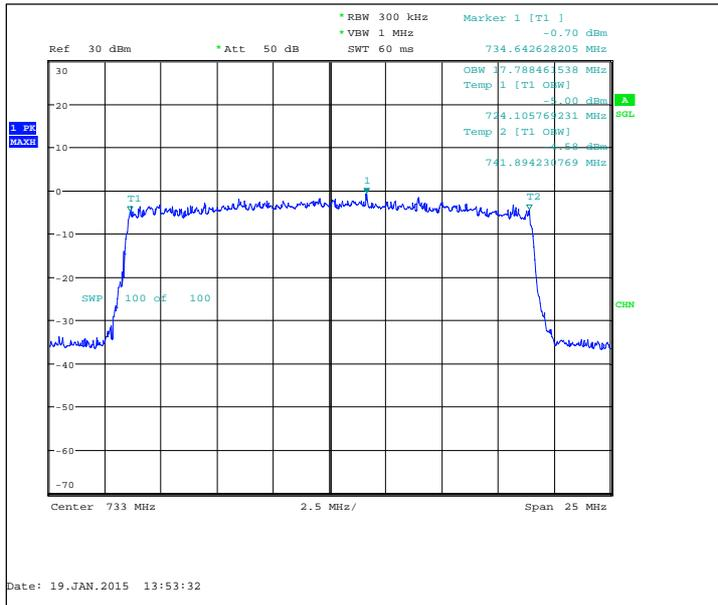
FDD, CBW 3MHz, 16QAM, 15 RB, Channel 27435 / 725.5 MHz
