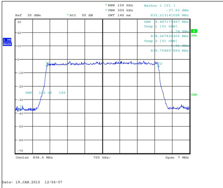
FDD, CBW 10MHz, 16QAM, 50 RB, Channel 20525 / 836.5 MHz
