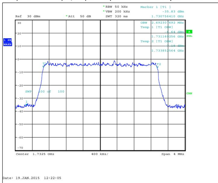
FDD, CBW 5MHz, QPSK, 25 RB, Channel 20175 / 1732.5 MHz
