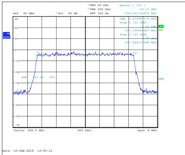
FDD, CBW 5MHz, 16QAM, 25 RB, Channel 20525 / 836.5 MHz
