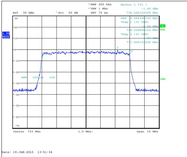
FDD, CBW 15MHz, QPSK, 75 RB, Channel 27435 / 725.5 MHz
