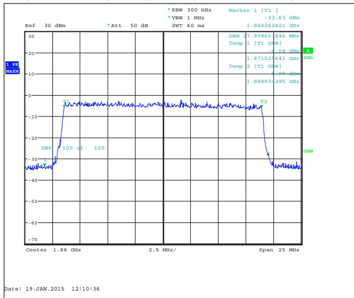
FDD, CBW 1.4MHz, 16QAM, 6 RB, Channel 18900 / 1880.0 MHz
