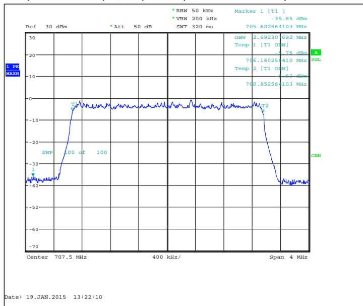
FDD, CBW 5MHz, QPSK, 25 RB, Channel 23095 / 707.5 MHz
