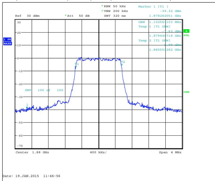
FDD, CBW 3MHz, QPSK, 15 RB, Channel 18900 / 1880.0 MHz
