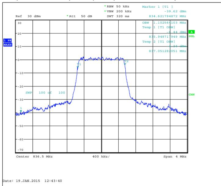
FDD, CBW 3MHz, QPSK, 15 RB, Channel 20525 / 836.5 MHz
