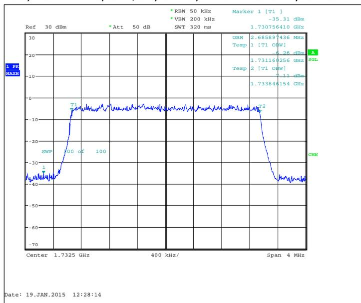
FDD, CBW 5MHz, 16QAM, 25 RB, Channel 20175 / 1732.5 MHz
