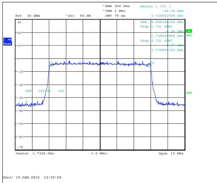
FDD, CBW 15MHz, 16QAM, 75 RB, Channel 20175 / 1732.5 MHz
