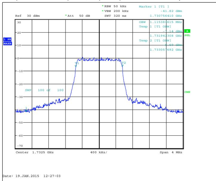
FDD, CBW 3MHz, 16QAM, 15 RB, Channel 20175 / 1732.5 MHz
