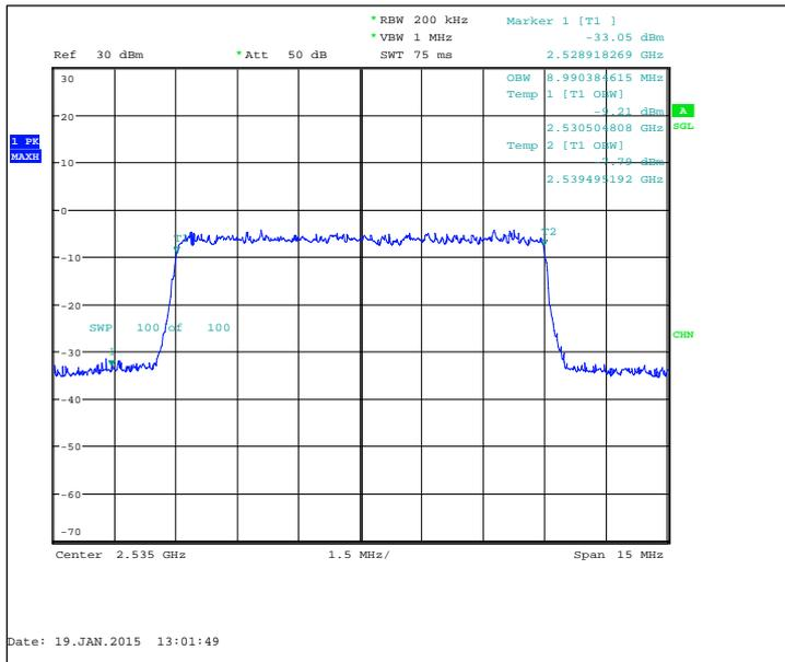
FDD, CBW 15MHz, QPSK, 75 RB, Channel 21100 / 2535.0 MHz
