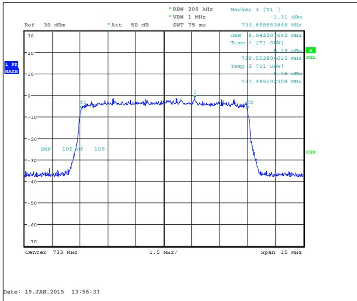
FDD, CBW 15MHz, 16QAM, 75 RB, Channel 27435 / 725.5 MHz
