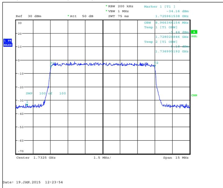
FDD, CBW 15MHz, QPSK, 75 RB, Channel 20175 / 1732.5 MHz
