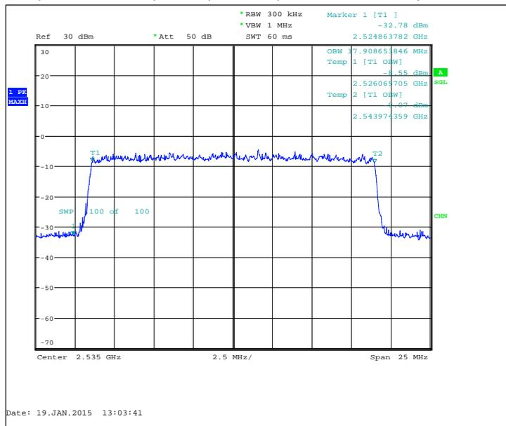
FDD, CBW 5MHz, 16QAM, 25 RB, Channel 21100 / 2535.0 MHz
