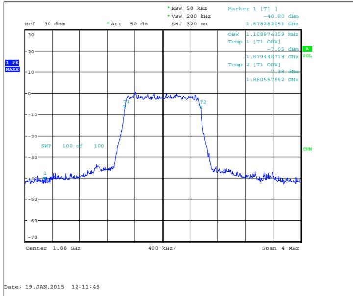
FDD, CBW 3MHz, 16QAM, 15 RB, Channel 18900 / 1880.0 MHz
