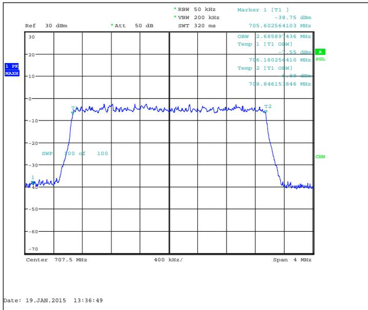
FDD, CBW 5MHz, 16QAM, 25 RB, Channel 23095 / 707.5 MHz
