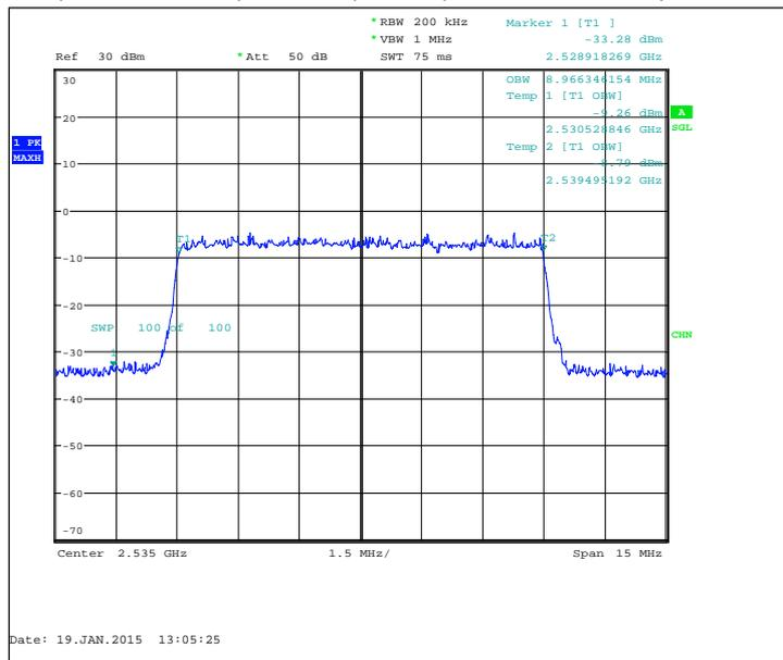
FDD, CBW 15MHz, 16QAM, 75 RB, Channel 21100 / 2535.0 MHz
