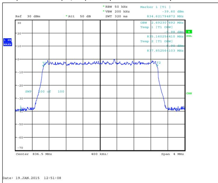
FDD, CBW 5MHz, QPSK, 25 RB, Channel 20525 / 836.5 MHz
