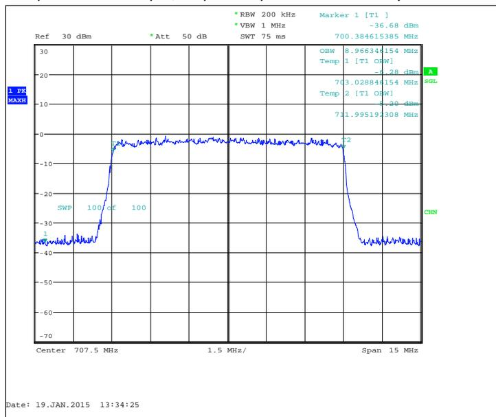
FDD, CBW 1.4MHz, 16QAM, 6 RB, Channel 23095 / 707.5 MHz
