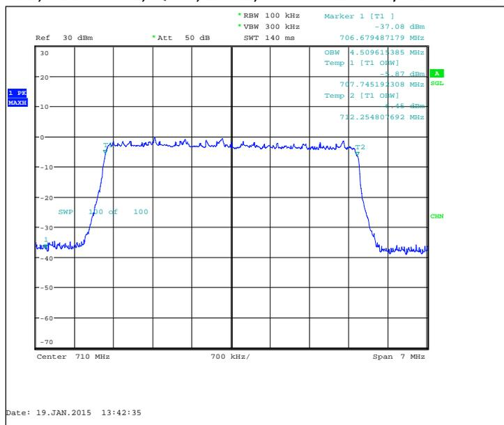
FDD, CBW 10MHz, QPSK, 50 RB, Channel 23790 / 710.0 MHz
