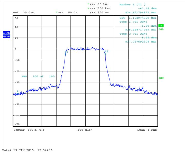
FDD, CBW 3MHz, 16QAM, 15 RB, Channel 20525 / 836.5 MHz
