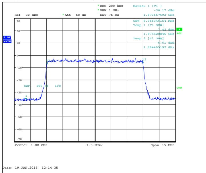
FDD, CBW 15MHz, 16QAM, 75 RB, Channel 18900 / 1880.0 MHz
