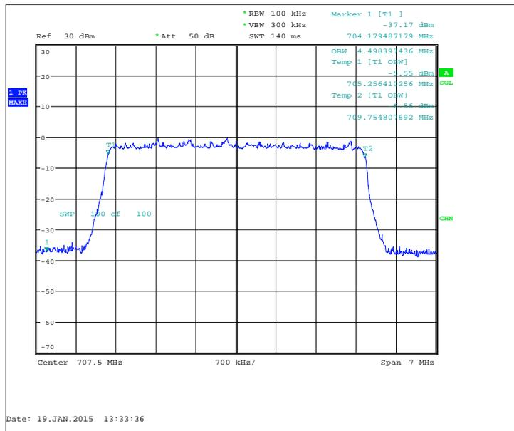
FDD, CBW 10MHz, QPSK, 50 RB, Channel 23095 / 707.5 MHz
