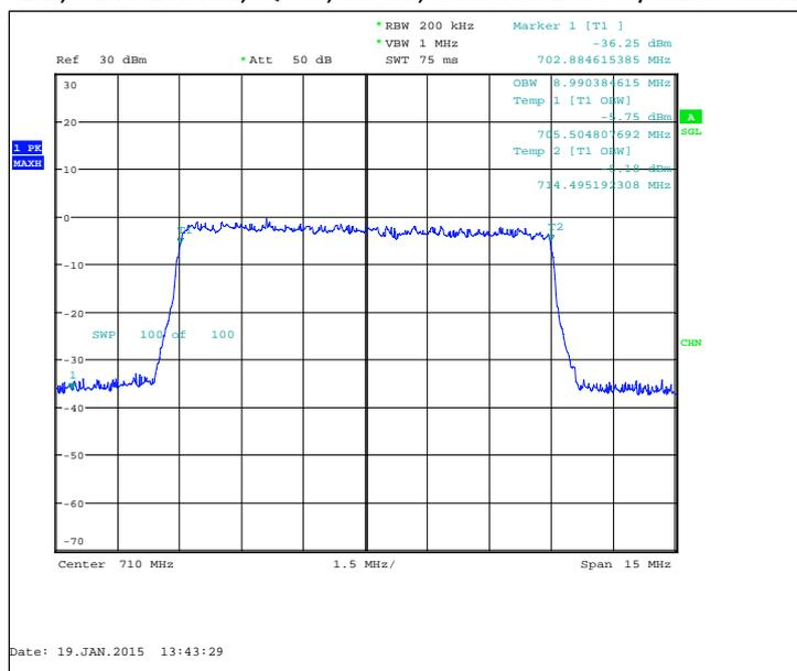
FDD, CBW 5MHz, 16QAM, 25 RB, Channel 23790 / 710.0 MHz
