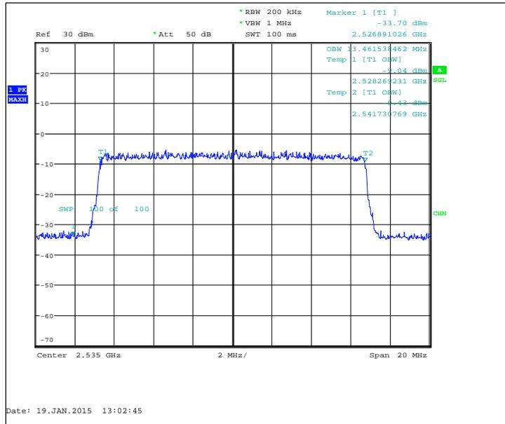
FDD, CBW 20MHz, QPSK, 100 RB, Channel 21100 / 2535.0 MHz
