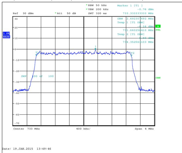
FDD, CBW 5MHz, QPSK, 25 RB, Channel 27435 / 725.5 MHz
