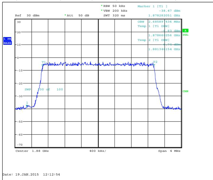
FDD, CBW 5MHz, 16QAM, 25 RB, Channel 18900 / 1880.0 MHz
