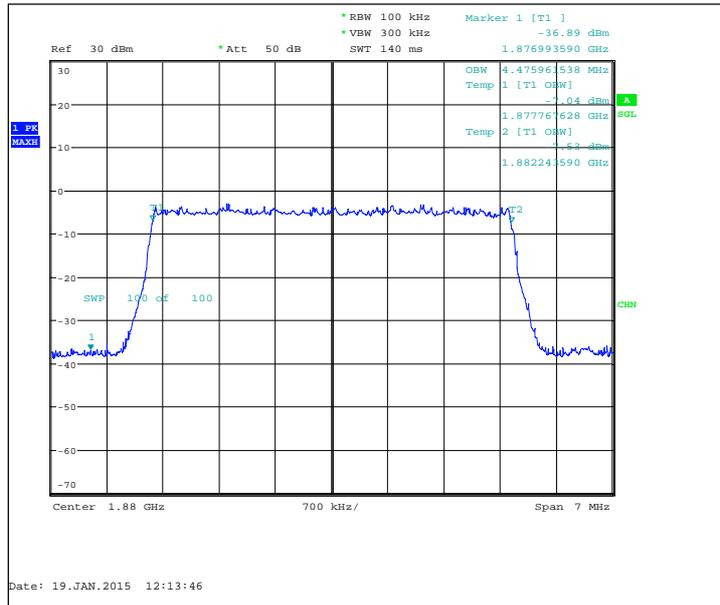
FDD, CBW 10MHz, 16QAM, 50 RB, Channel 18900 / 1880.0 MHz
