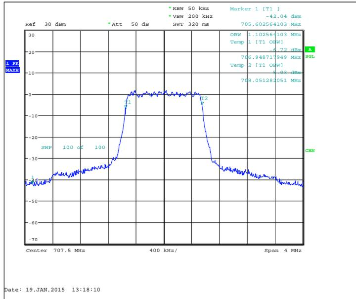
FDD, CBW 3MHz, QPSK, 15 RB, Channel 23095 / 707.5 MHz
