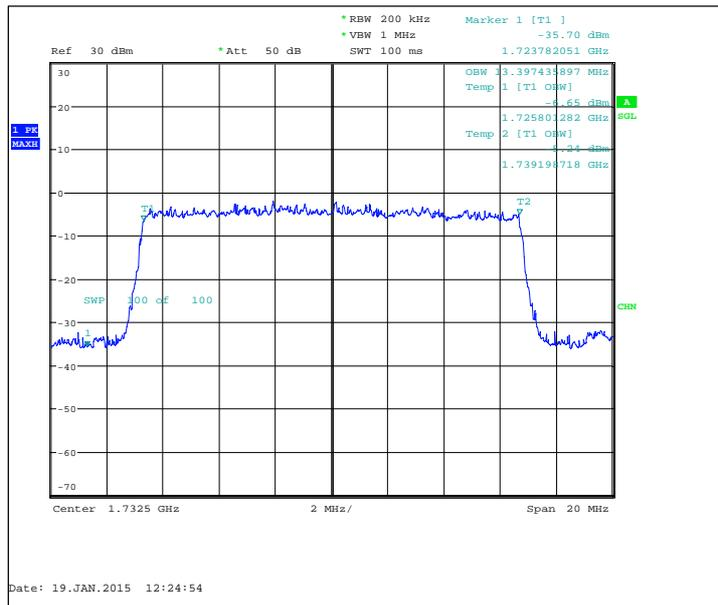
FDD, CBW 20MHz, QPSK, 100 RB, Channel 20175 / 1732.5 MHz
