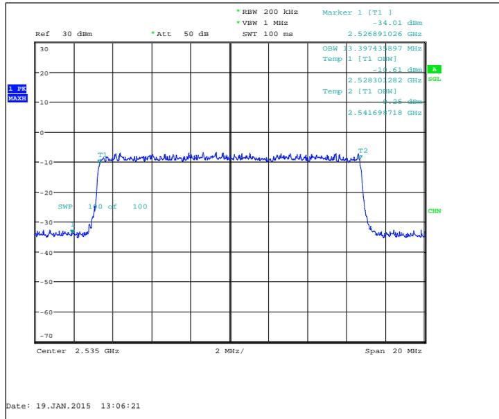
FDD, CBW 20MHz, 16QAM, 100 RB, Channel 21100 / 2535.0 MHz
