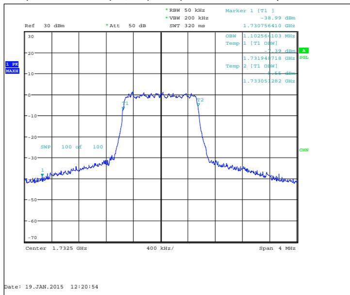
FDD, CBW 3MHz, QPSK, 15 RB, Channel 20175 / 1732.5 MHz
