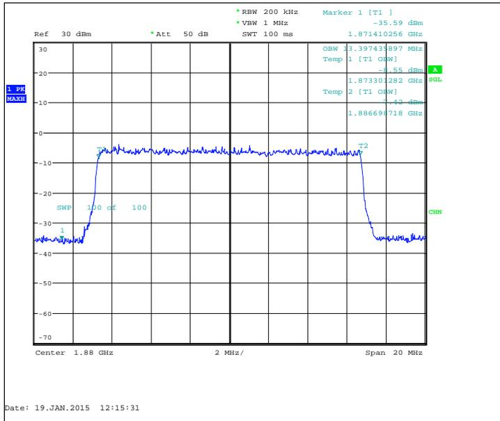
FDD, CBW 20MHz, 16QAM, 100 RB, Channel 18900 / 1880.0 MHz
