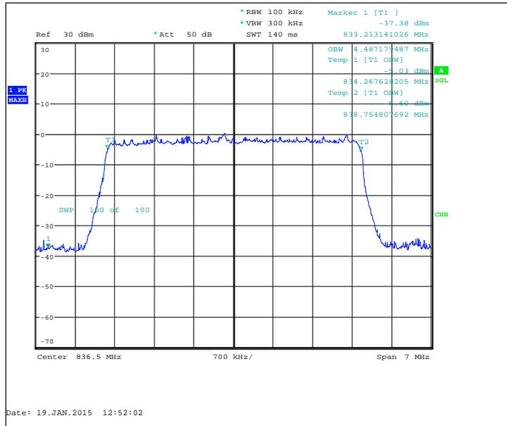
FDD, CBW 10MHz, QPSK, 50 RB, Channel 20525 / 836.5 MHz
