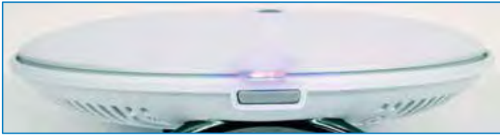
Figure 4: Purple LED – Booster is syncing
