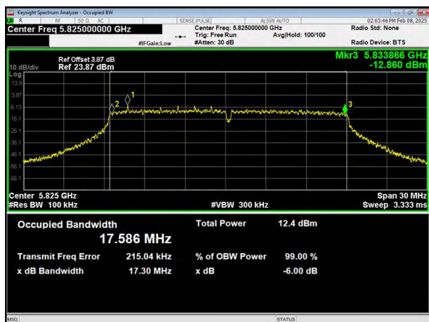
(802.11n20) 6dB Bandwidth plot on channel 165
