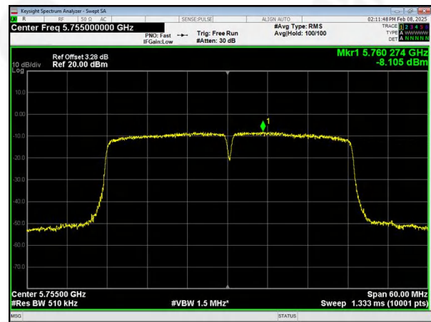
(802.11ac40) PSD plot on channel 159
