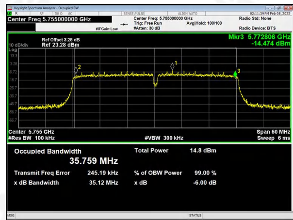
(802.11ac40) PSD plot on channel 151
