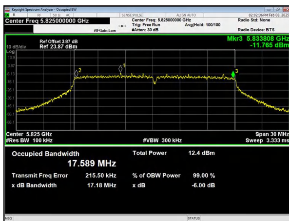
(802.11ac20) 6dB Bandwidth plot on channel 165
