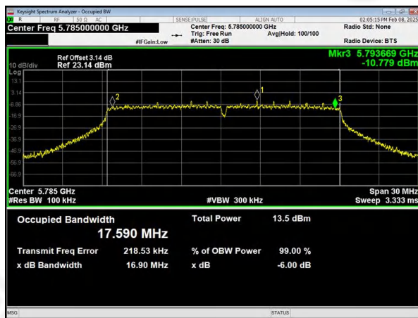
(802.11ac20) 6dB Bandwidth plot on channel 165
