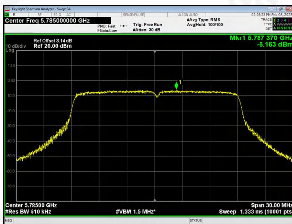
(802.11ac20) PSD plot on channel 157
