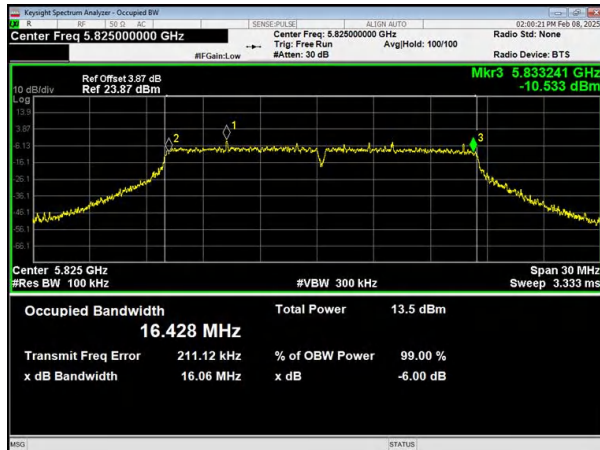
(802.11a) 6dB Bandwidth plot on channel 165
