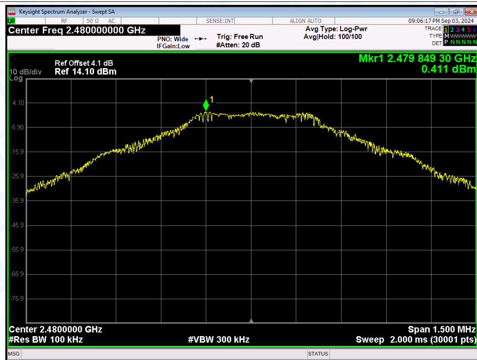
Tx. Spurious NVNT 1-DH1 2480MHz Ant1 Emission
