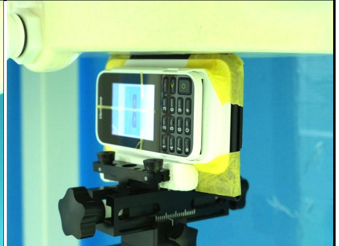
Limb - Right Side of EUT at 0 mm
