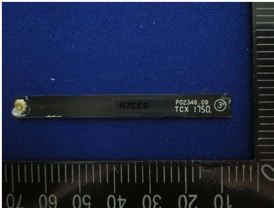
EUT –RF Ant 1 Top View
