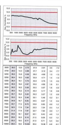
Figure J-3 600 – 10000 MHz Head Tissue Equivalent Matter
