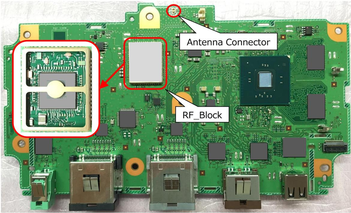
Fig.5 WLAN\_PCB (w/o Heat Sink) [Surface-Side]
