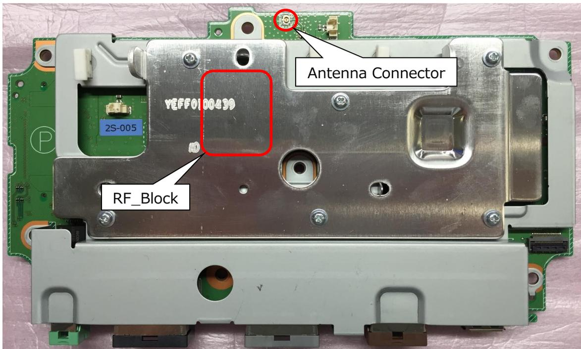
Fig.4 WLAN\_PCB (w/ Heat Sink) [Surface-Side]
