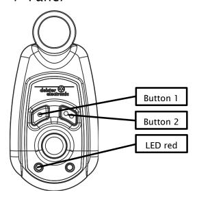
The panel of the tag consists of three buttons and and two LEDs.
