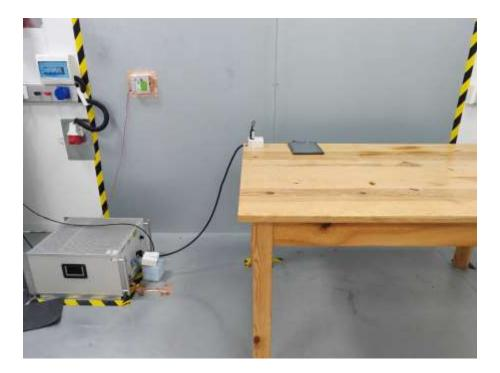
Set-up for Radiated Emission (RE), Below 1GHz
