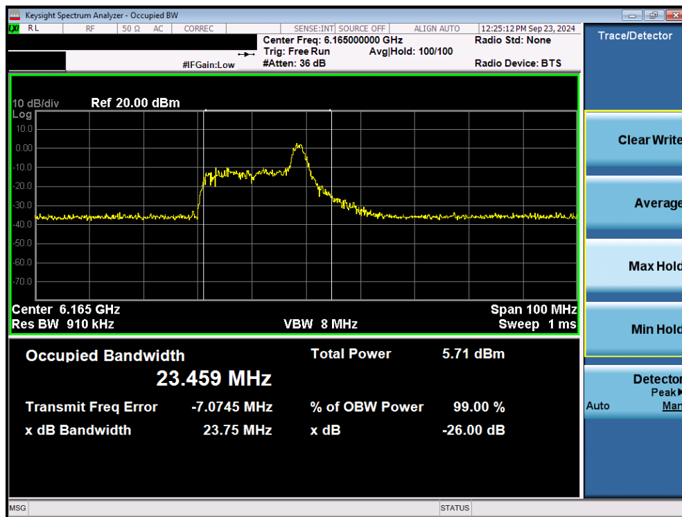
Plot 7-9. 26dB Bandwidth Plot MIMO ANT1 (40MHz 802.11ax/be (26 Tones) (UNII Band 5) – Ch. 43) - VLP
