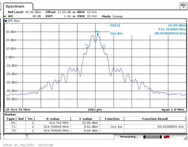
99% Occupied Bandwidth Plot on 914.75 MHz
