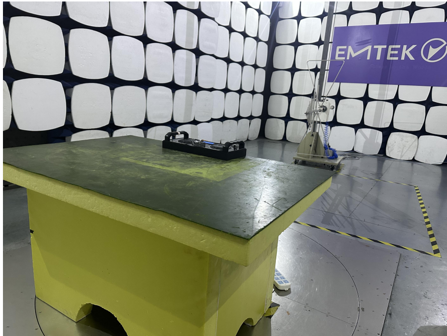
Spurious Emission Test Setup (Above 1GHz)
