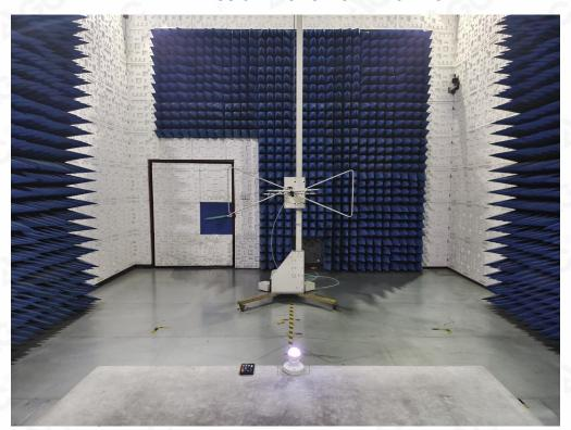
RADIATED EMISSION TEST SETUP ABOVE 1GHz
