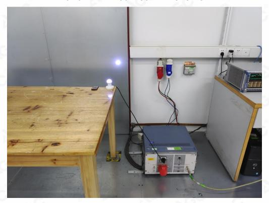
RF CONDUCTED TEST SETUP
