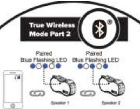
Once both speakers are in True Wireless mode, they will automatically pair with a Bluetooth-enabled device.
