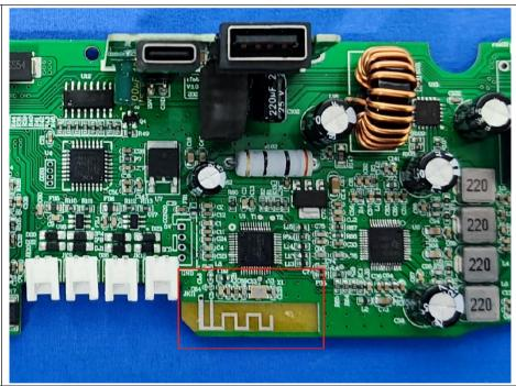
The antenna is PCB antenna. The best case gain of the antenna is 3.38 dBi.
