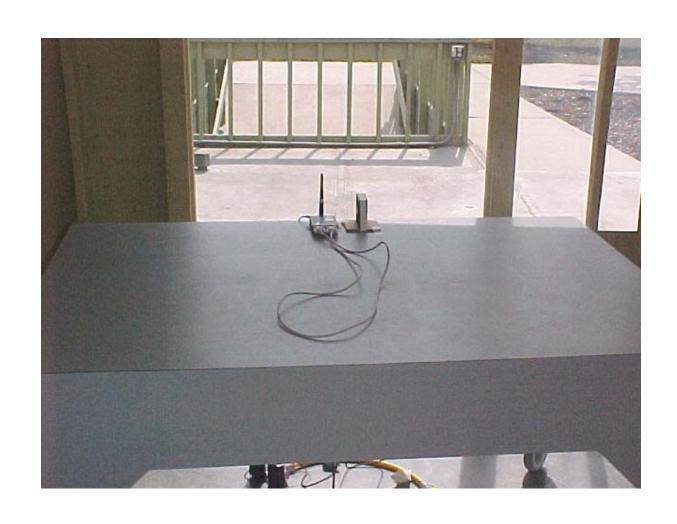
Radiated Emissions Measurement (Front View) Setup
