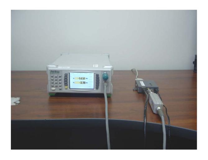
Maximum Peak Output Power Measurement Setup
