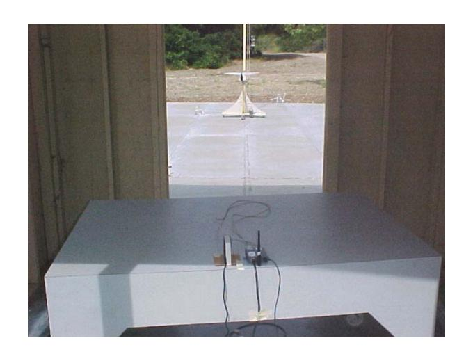
Radiated Emissions Measurement (Rear View) Setup
