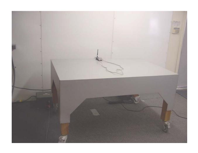
AC Conducted Emissions Measurement (Front View) Setup
