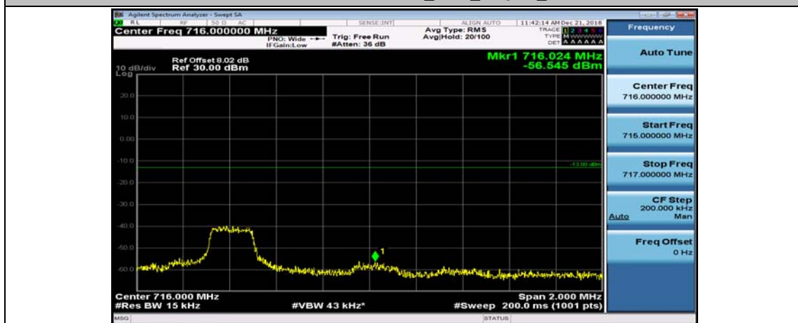
Channel Bandwidth: 10 MHz_HCH_16QAM_1RB#24
