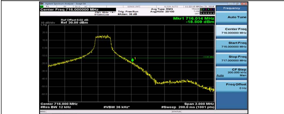
(Channel Bandwidth: 5 MHz)_HCH_16QAM_12RB#0
