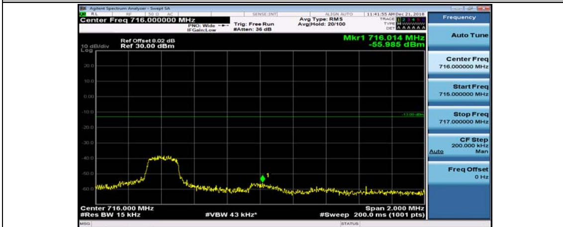
Channel Bandwidth: 10 MHz_HCH_QPSK_1RB#24
