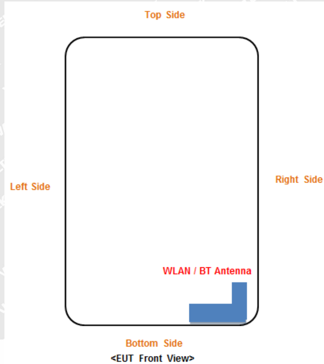
Fig 7.1 Block Diagram for EUT Antenna Position EUT Size: Long*Width*Height=20.9cm*12.5cm*1.0cm
