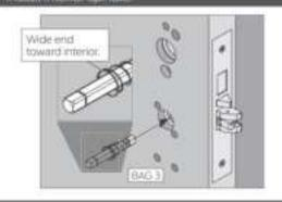
Bb. Route cables and posts though holes as shown. Push assembly against door and hold.
