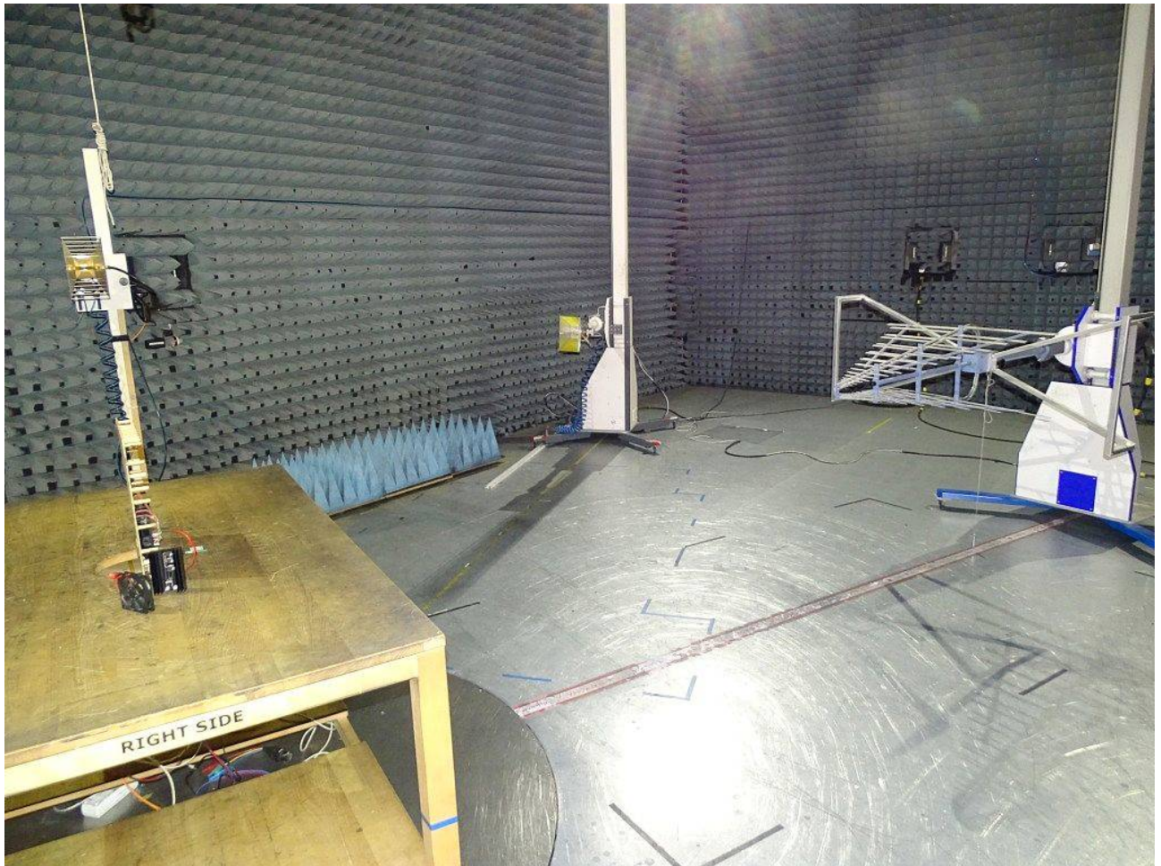
Photo 3: Test setup for radiated measurements (Enclosure, semi-anechoic chamber, 30 MHz to 1 GHz, intentional radiator §15, ANSI C63.10) WPT
