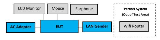
3.10.2. EUT Configuration for RF Conducted Test Items
