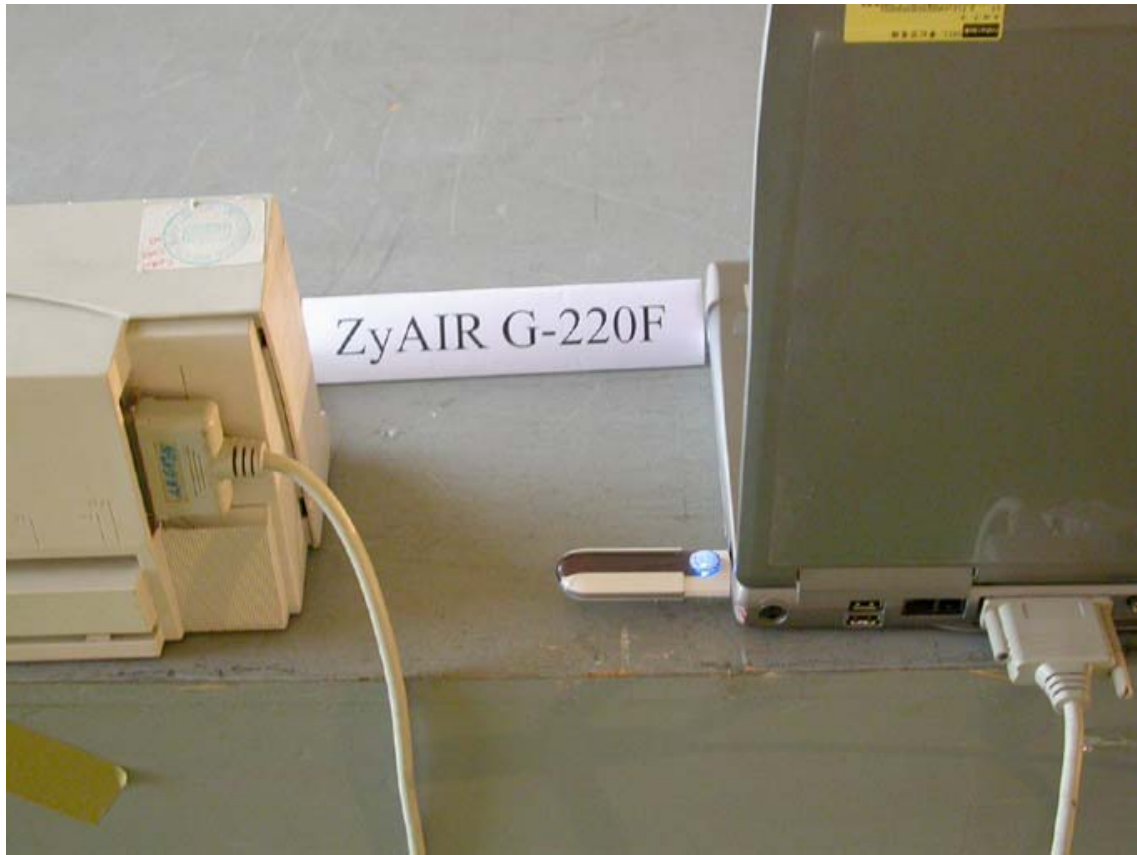
Photo 3: Radiated Emission Test set-up photo
