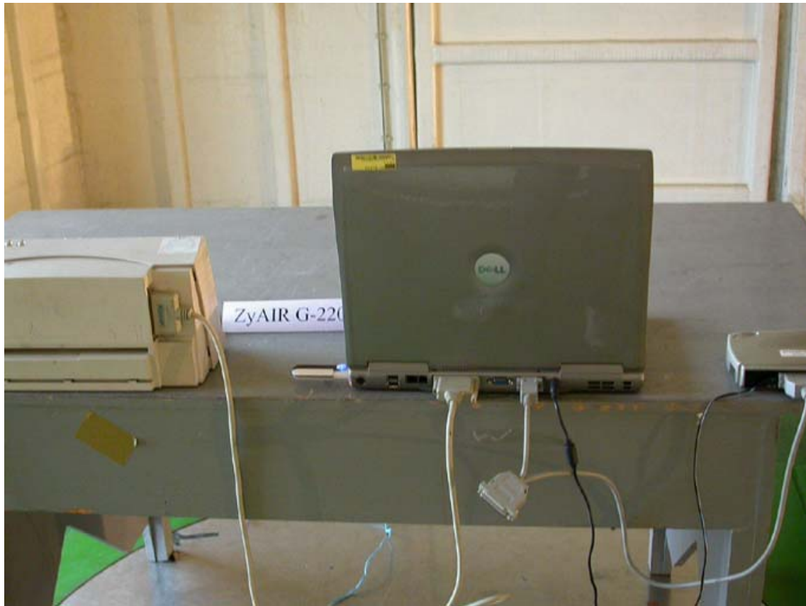
Photo 3: Radiated Emission Test set-up photo
