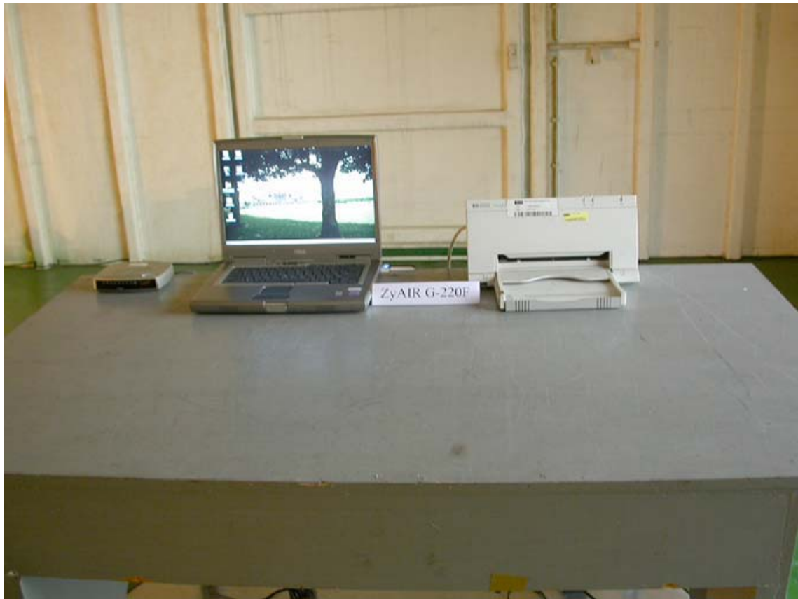
Photo 1: Radiated Emission Test set-up photo
