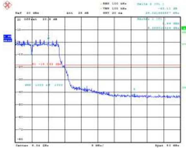
Figure 7-33: Band Edge Compliance Primary, 802.11a, Channel 64, 6 Mbps
