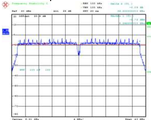
Figure 8-17: 6 dB Bandwidth Secondary, 802.11ac, Channel 64, 6 Mbps
