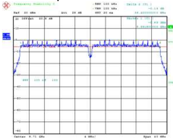
Figure 8-19: 6 dB Bandwidth Secondary, 802.11ac, Channel 140, MCS0 Mbps
