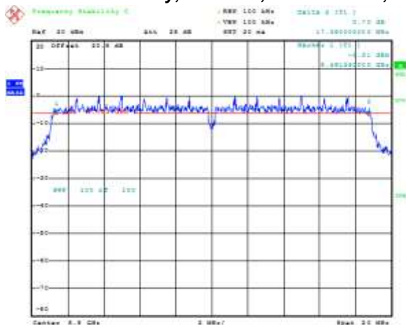
Figure 8-3: 6 dB Bandwidth Primary, 802.11ac, Channel 100, 6 Mbps
