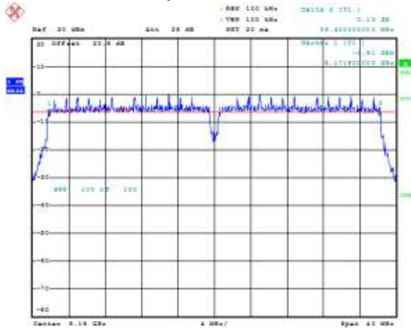
Figure 7-23: 6 dB Bandwidth Primary, 802.11n, Channel 36, MCS 0
