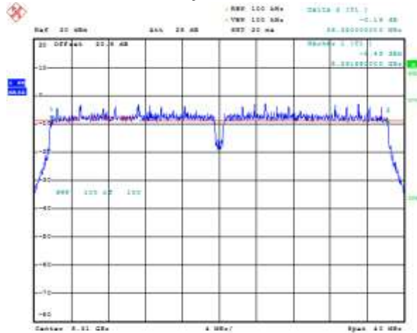
Figure 7-24: 6 dB Bandwidth Primary, 802.11n, Channel 64, MCS 0
