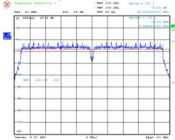
Figure 8-12: 6 dB Bandwidth Primary, 802.11ac, Channel 64, MCS0 Mbps
