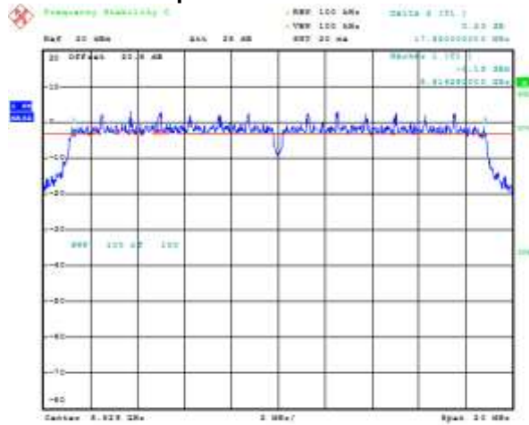
Figure 8-10: 6 dB Bandwidth Secondary, 802.11ac, Channel 149, MCS0 Mbps
