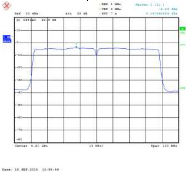
Figure 8-100 Peak Power Spectral Density SISO Secondary, 802.11ac, Channel 42, MCS0 Mbps
