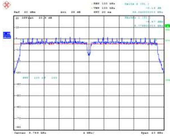
Figure 7-27: 6 dB Bandwidth Primary, 802.11n, Channel 161, MCS 0
