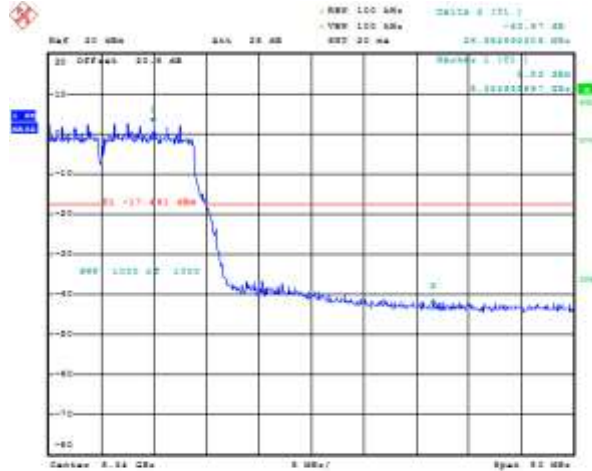
Figure 7-45: Band Edge Compliance Primary, 802.11n, Channel 64, 6 Mbps
