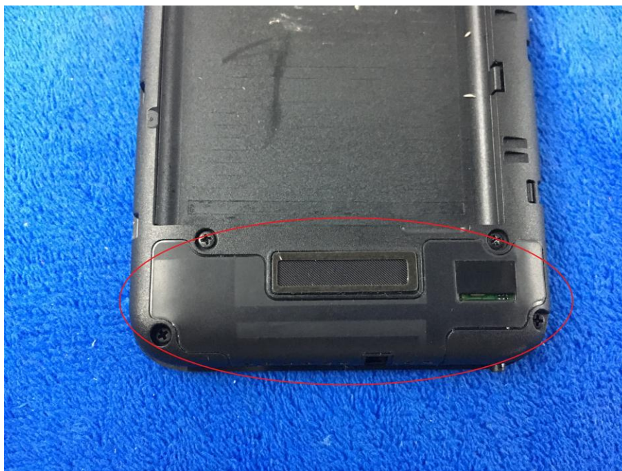
GSM/PCS/UMTS - Antenna View
