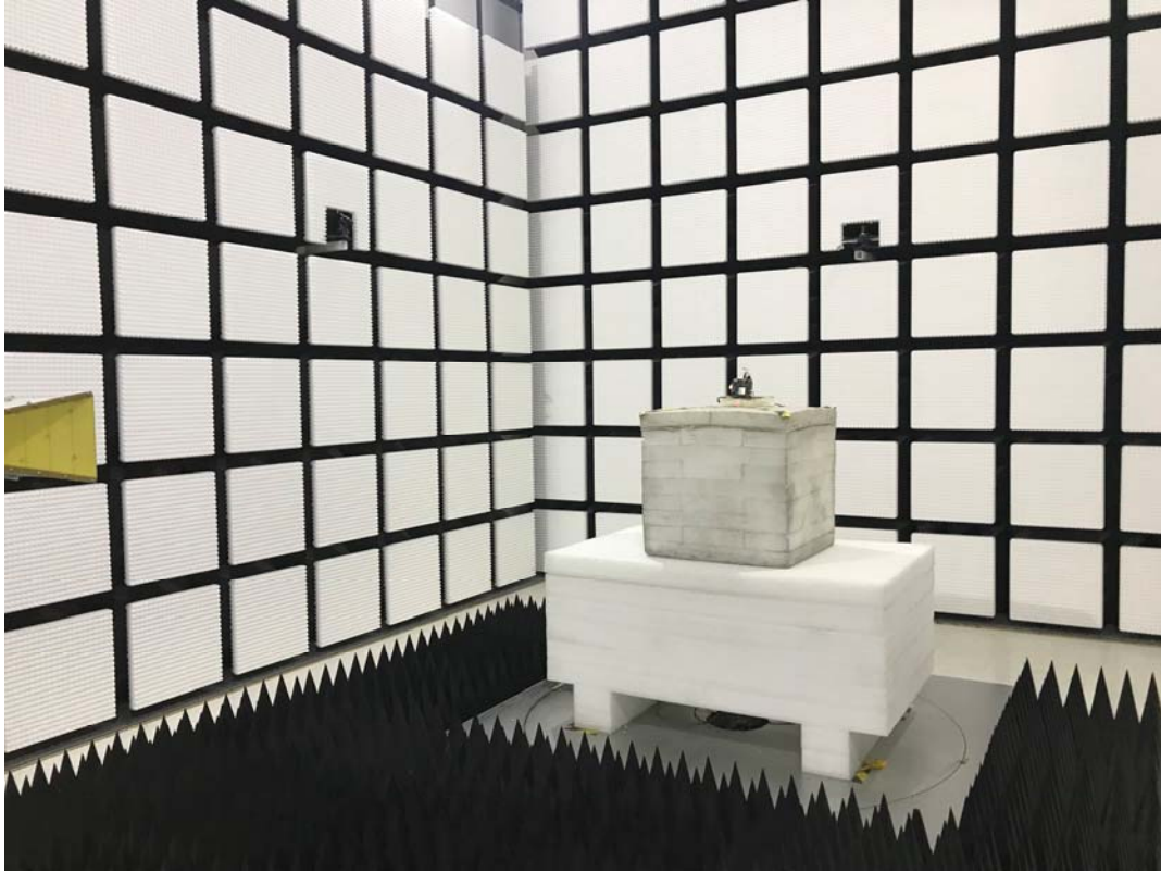
Radiated Emissions Above 1G View-FPC Antenna
