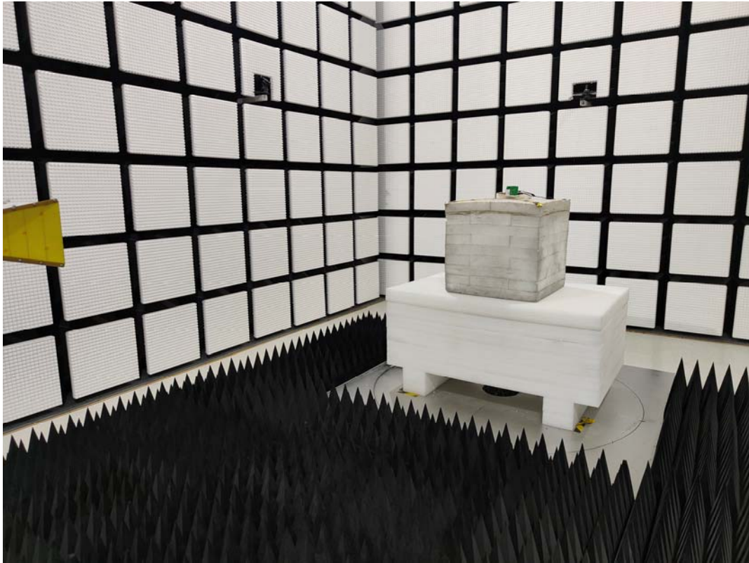
Radiated Emissions Above 1G View-PCB Antenna
