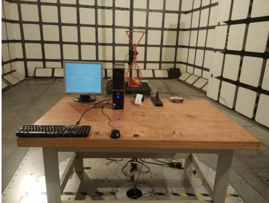
Radiated Emissions – Front View (Below 1 GHz)
