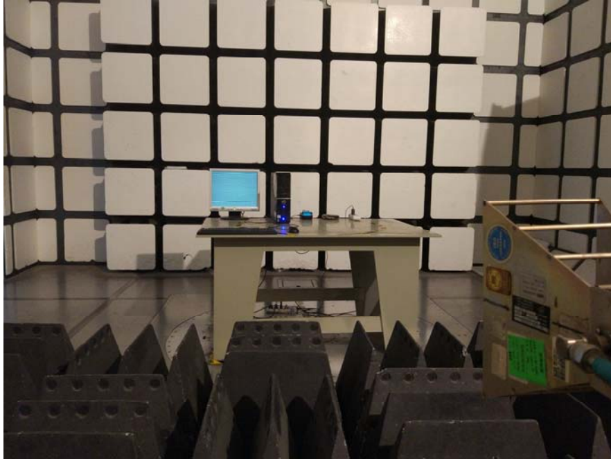
Radiated Emissions – Front View (Above 1 GHz)
