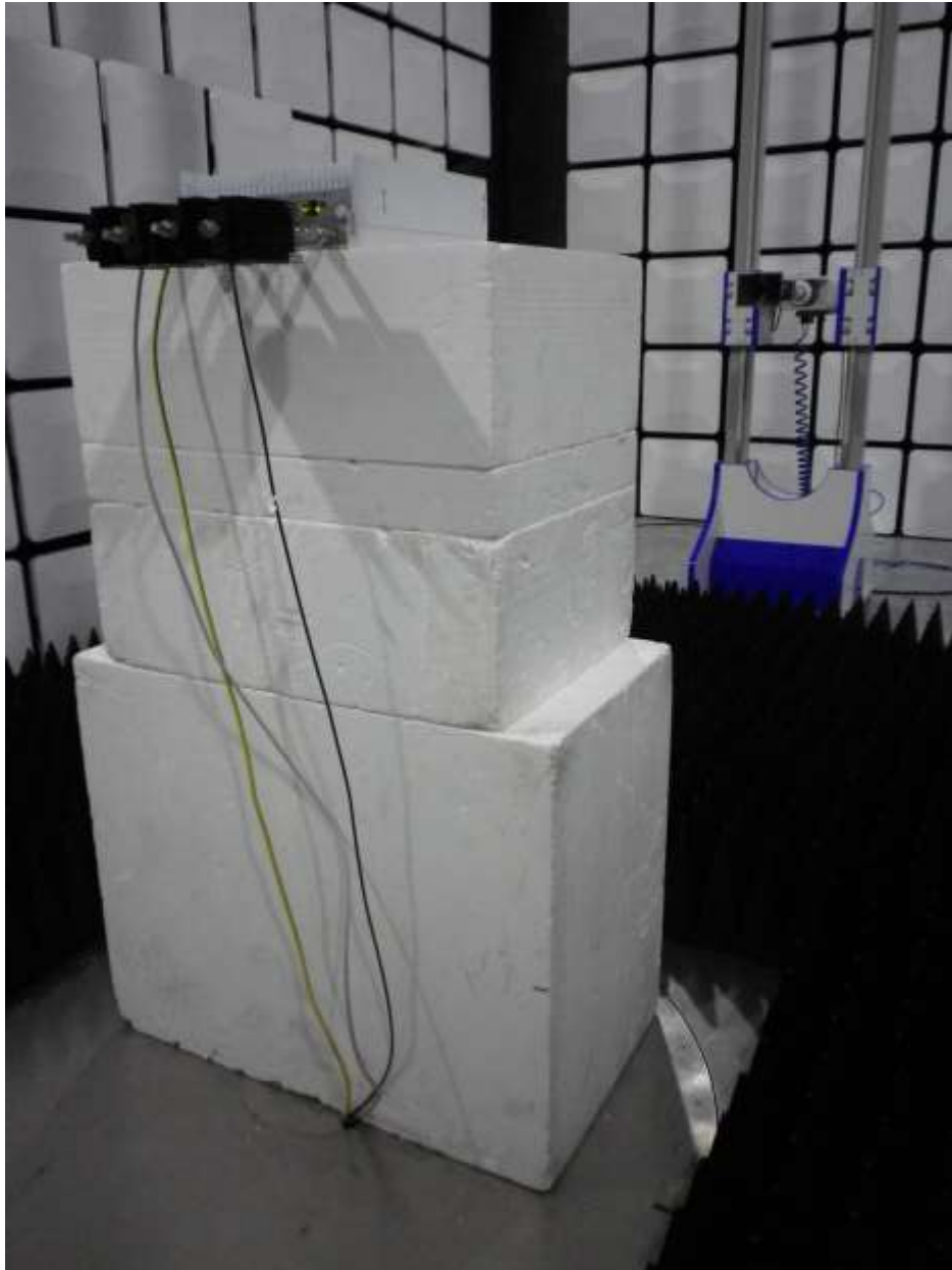
Radiated 1GHz – 18GHz Testing
