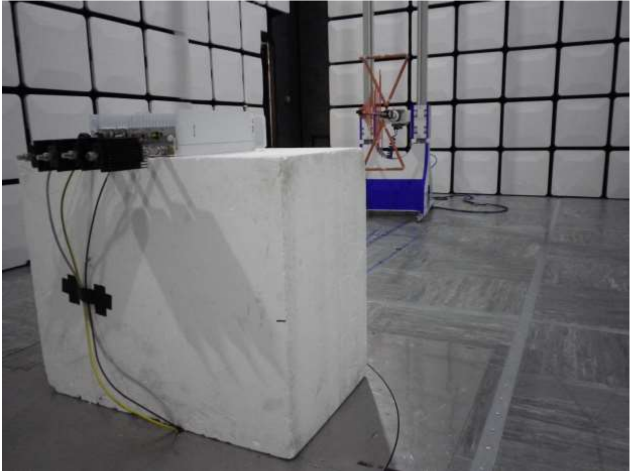
Radiated 30 MHz – 1GHz Testing
