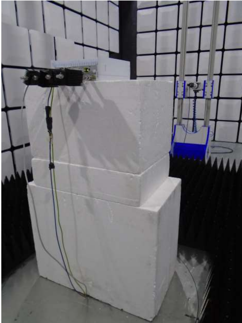
Radiated 18GHz – 22GHz Testing
