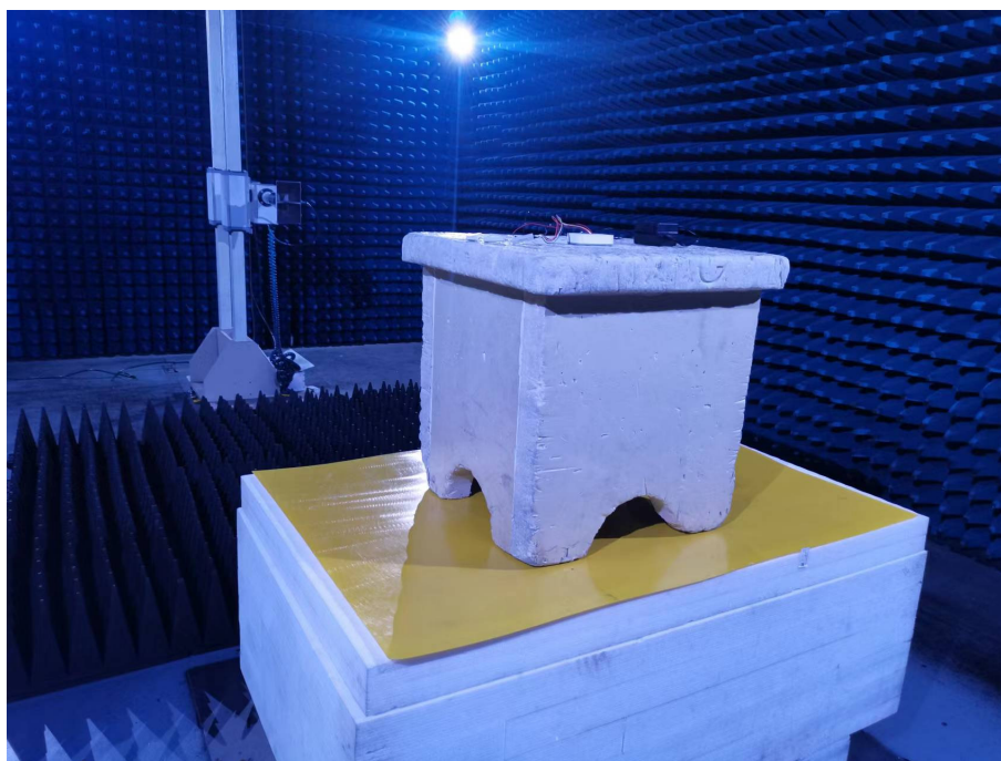
Photo of Radiated Emission Measurement (Above 1G)
