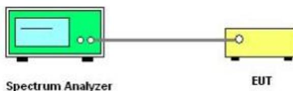
The EUT is connected to the Spectrum Analyzer; the RF load attached to the EUT antenna terminal is 50Ohm; the path loss as the factor is calibrated to correct the reading. Make the measurement with the spectrum analyzer's resolution bandwidth (RBW) = 100 kHz. In order to make an accurate measurement, set the span greater than RBW.
