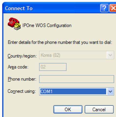
Fig. 3.2.2 HyperTerminal Select modem port
