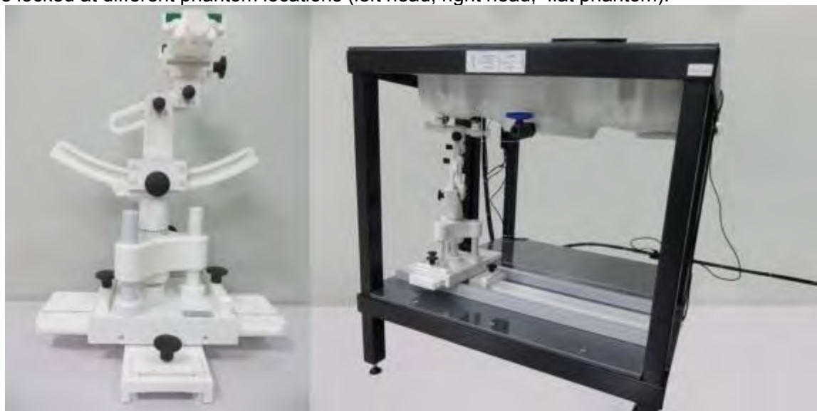
Device holder supplied by SATIMO
