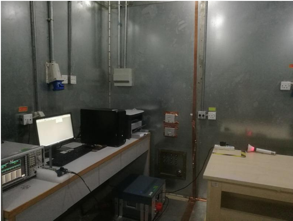
FCC RADIATED EMISSION TEST SETUP
