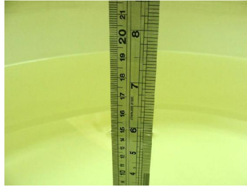
Fig 7.2 Photo of Liquid Height for Body SAR
