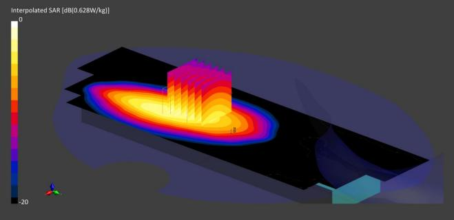
Communication System: CW UID: 0; Frequency: 927.6 MHz; Duty Cycle: 1;
